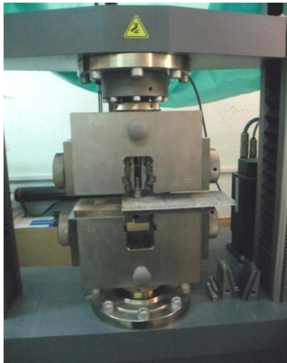
Figure 3.2: La machine de traction-compression Zwick/Roell.
